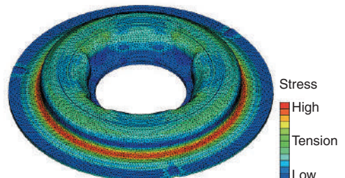
Under load (stress distribution diagram)
