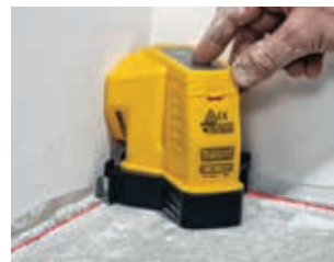
Positions inside corners to check for square
