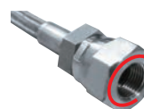
nut G1/8 internal thread Fix by rotating nut (No need to rotate hose)
