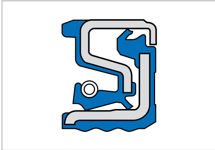
Fig.1 Simmerring Cassette Seal Type 1
