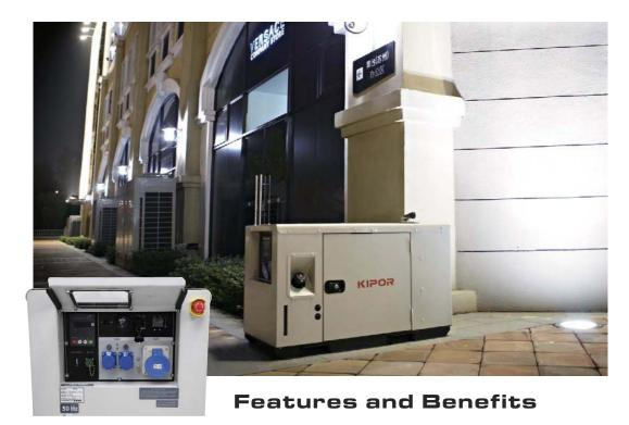
The permanent magnet alternator eliminates excitation windings, carbon brushes and rotor slip rings. The construction is much simpler with the stator bolted directly to the engine. The alternator is smaller in size but can achieve an alternator efficiency of 93%. High in reliability, free of radio interference and capable of operating in high humidity and dusty environments.
