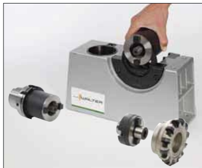
5. Insert the extension into the retaining collar.
