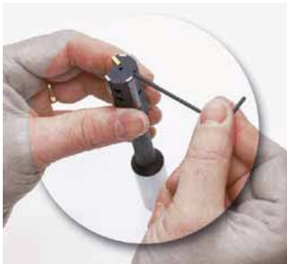
1. Slacken the 2 adjusting screws ① by rotating them anticlockwise by 1/4 of a turn.
