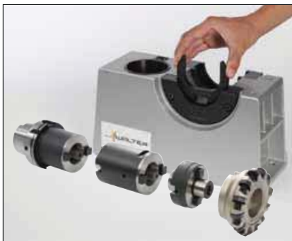
4. Insert the retaining collar V 530 into the flange V 510.10.050.
