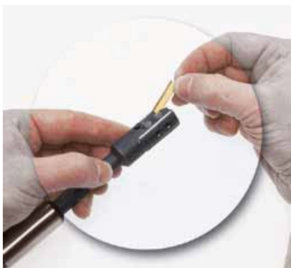
3. Thoroughly clean the insert seat and the insert. Turn the insert ④ or insert a new one.
