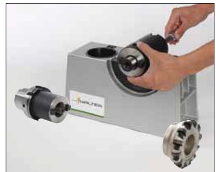
6. Screw the extension and the cutter adaptor together by hand using the extended socket key.
