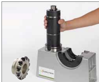
11. Insert the assembled adaptors into the tapered bush.
