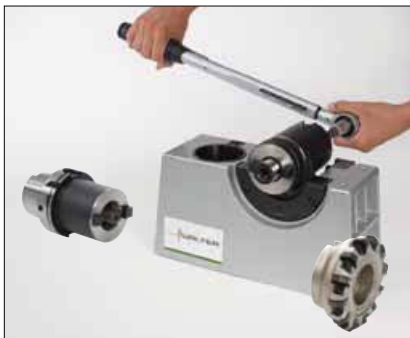
7. Tighten with a torque wrench.
