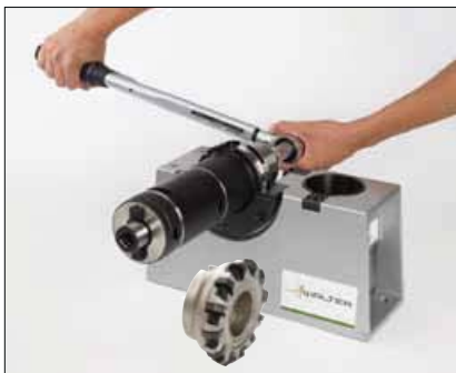
10. Tighten with a torque wrench.
