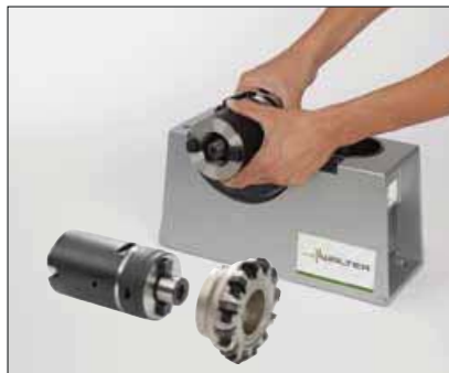
8. Insert the master into the associated flange.
