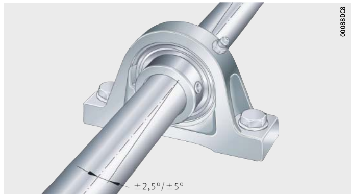
Figure 1 Compensation of static shaft misalignment
