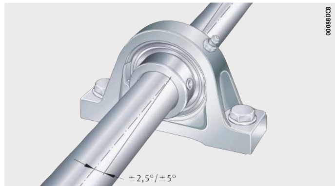
Figure 1 Compensation of static shaft misalignment
