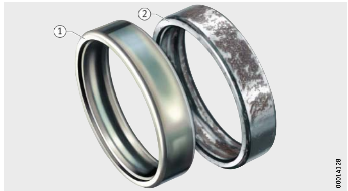
Figure 7 Bearing rings after the salt spray test
