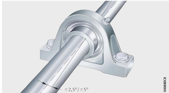
Figure 5 Compensation of static shaft misalignment
